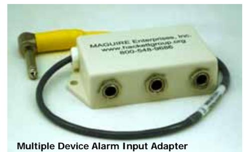
MAGUIRE Enterprises, Inc. manufactures a comprehensive line of medical interconnect cables which include Device Nurse Call Alarm cables to connect monitoring and therapy devices to your existing device alarm nurse call system.
