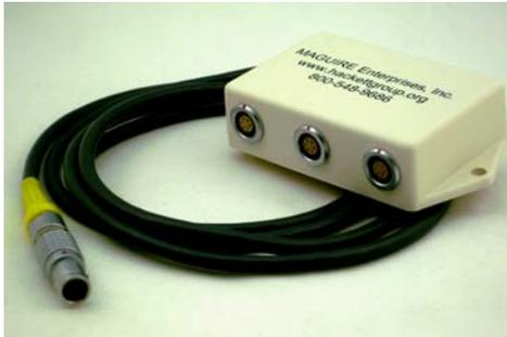
An output multiplier that 'reproduces' the output connector three times.
